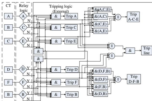
Figure 6. External trip logic for a six-phase transmission line protection.
