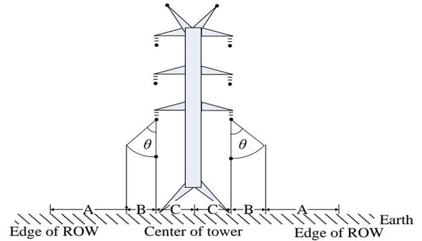
Figure 3. Transmission line right-of-way
