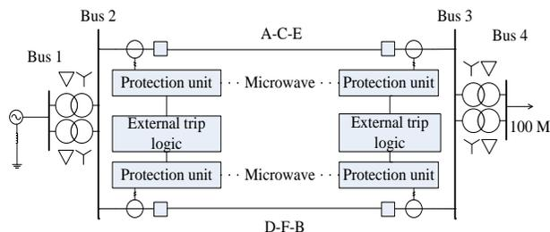
Figure 7. External trip logic for a six-phase transmission line protection.
