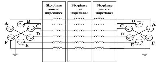
Figure 5. Six-phase equivalent system network.
