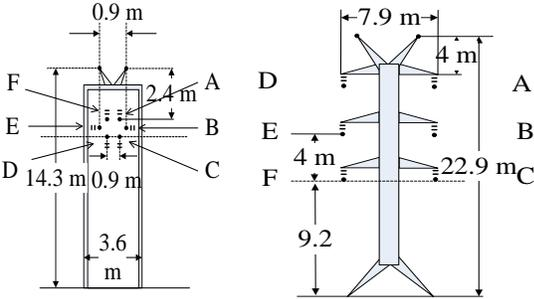
Case 3: 80 kV six-phase compact tower transmission line
