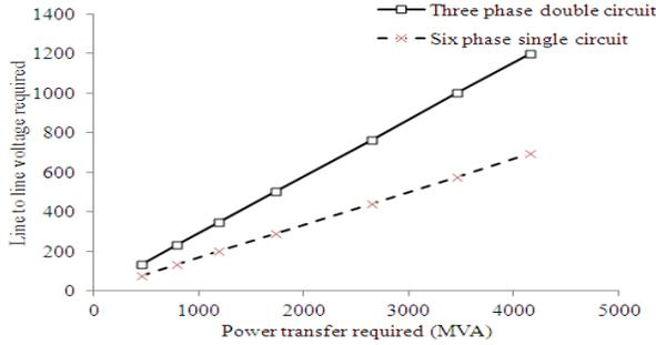
Figure 4. Voltage requirements for three phase double circuit and six-phase single circuit for same amount of power transfer
