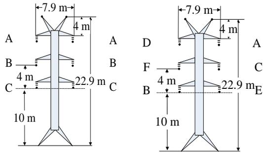
Case 1: 138 kV three-phase double circuit conventional tower line
