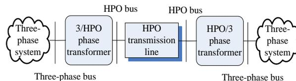
Figure 1. Three-phase system and high phase order transmission line connection diagram.
